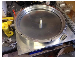
Figure 9 Final aluminium mould put together and polished
